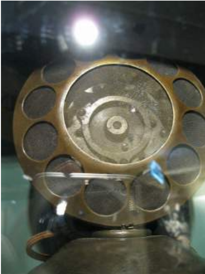
Western Electric Microphone, Model 387, Double Button Carbon Microphone, early 1920s. Together with the one developed by the Bell Laboratories, this microphone represents one of the decisive technological advances in the history of sound recording. Birthplace of Country Music Museum, Bristol VA. Photo: G. De Smaele, 2018.
